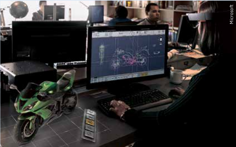
Microsoft's HoloLens augmented reality headset projects holographics into the line of vision, and allows the users to interact with content and information with movement and voice recognition
