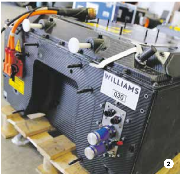
1. McLaren's motor generator unit powering the Formula E series 2. The 200kW batteries developed by Williams
