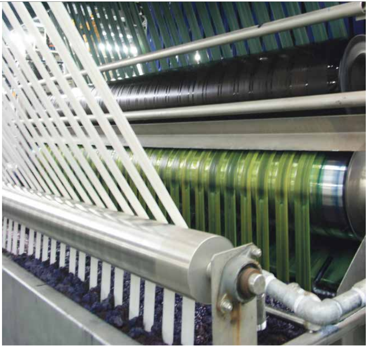
ISKO's high-tech machinery at work in the indigo dyeing process
