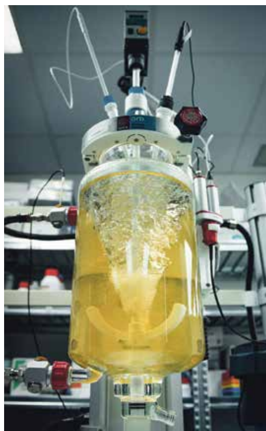
A mid-scale 10-litre reactor manufacturing Midatech's gold-core nanoparticles
